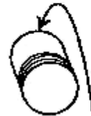
Cut back male end of one 50mm joiner (x2) so that only 5mm protrudes this will be the inside of urine outlet
